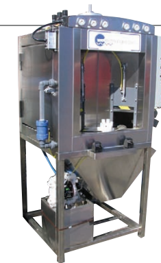
3000 psi high pressure closed loop water system (black box)
