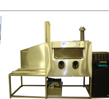
3000 psi high pressure closed loop water system (black box)
