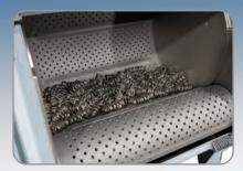
**Durable, continuous-molded rubber belt** tumbles parts within the blast envelope to assure uniform processing.
