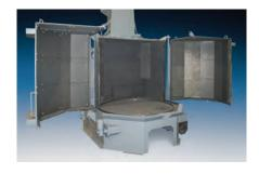
**96" XT Table Blaster**, designed to satisfy almost any part loading requirement, processes workpieces weighing up to 10,000 pounds with diameters to 96 inches and heights to 84 inches.
