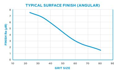
Testing conducted using 90 psi and 1018 carbon steel Angular media only.
