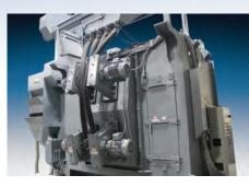
High-capacity blast machine performs both *Table* and *Spinner Hanger* operations, providing the versatility to meet various customer needs.
