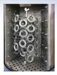
Gibson also offers custom fixture designs to maximize equipment efficiency.
