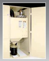
ProFormer™ cabinets are equipped with cartridge dust collectors to facilitate a quick change of filtration surfaces. These two cartridges have a filtration area of 103 square feet each, providing a total of 206 square feet, and can be replaced in minutes through the cabinet door. As a result, loose dust falls into the cabinet rather than onto the work floor.
