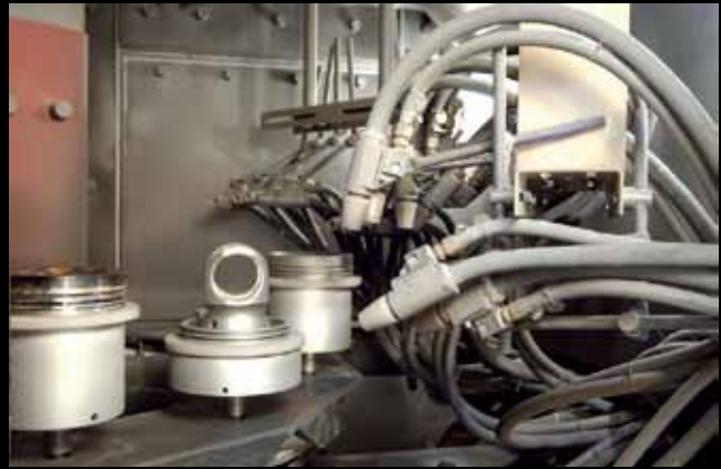
Indexing Turntable Machine coordinates 16 blast guns, oscillating vertically and horizontally, with rotating work stations to assure thorough cleaning in a single pass.
