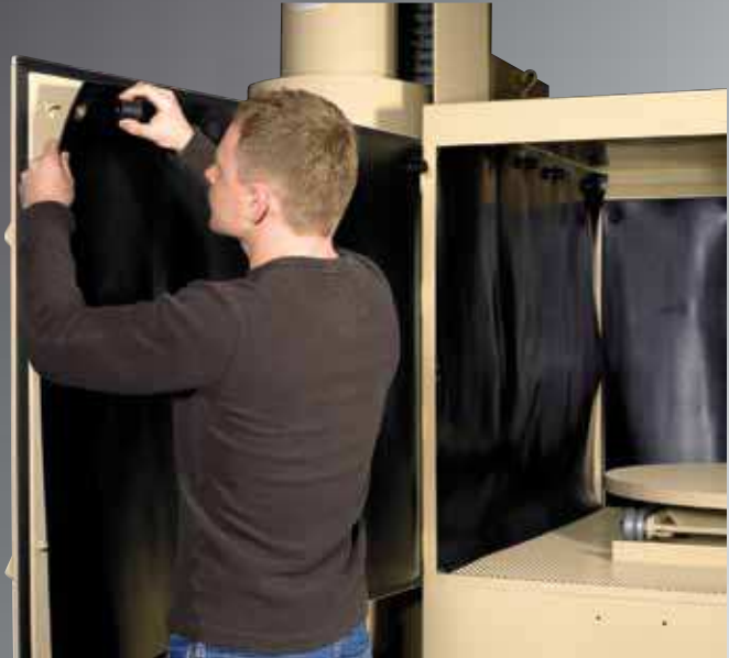
Rubber curtains , available in white to enhance visibility, protect cabinet interiors and are easy to replace.
