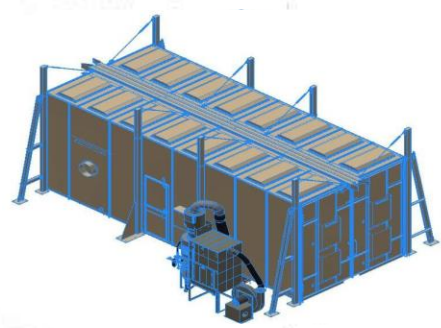
Drive Through Design with Crane Slot
