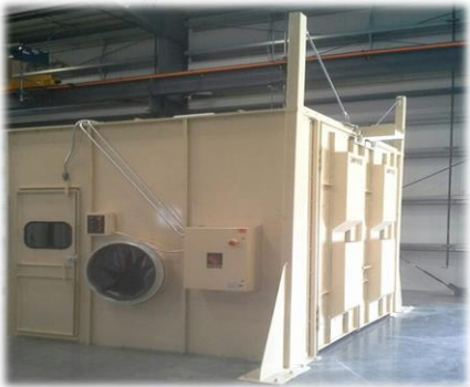
PEB Enclosure with Pipe Entry Vestibule
