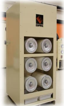
Booth Ventilation Dust Control Module connects to Enclosure End
