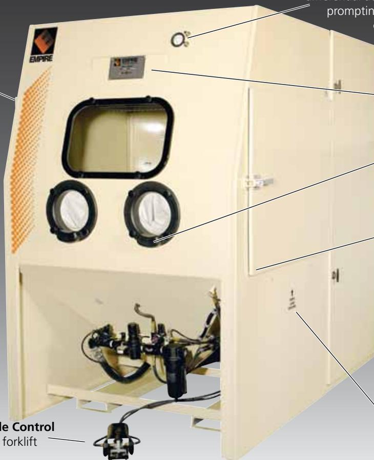
**Minihelic Gauge** shows the pressure differential across filtration surfaces, prompting the operator to pulse-clean dust-collector cartridges.
