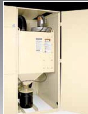
ProFormer™ cabinets are equipped with cartridge dust collectors to facilitate a quick change of filtration surfaces. These two cartridges have a filtration area of 103 square feet each, providing a total of 206 square feet, and can be replaced in minutes through the cabinet door. As a result, loose dust falls into the cabinet rather than onto the work floor.
