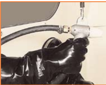
Empire MH-2 blast guns or pressure nozzles are available with tungsten carbide or silicon carbide to reduce wear with certain types of media.
