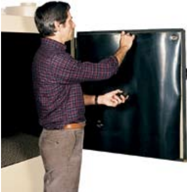
Rubber curtains, available in white to enhance visibility, protect the cabinet interior and are easy to replace.
