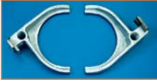
Shifter forks etched with ALOX
