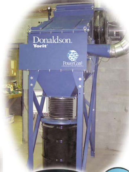
Torit PowerCore CPC-3 on clay and cement blending at a concrete block plant.
